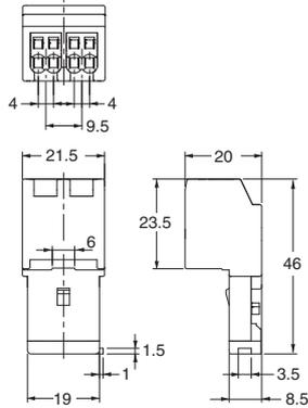
The contacts in this unit operate when the main unit trips due to an overload, phase failure, or short circuit.
