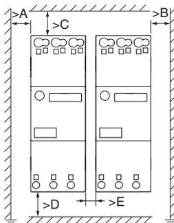
\* When units are closely mounted together, the thermal characteristics may change because of temperature increases due to the operating conditions (high ambient temperature or maximum set continuous carry current). If the unit operates unnecessarily, slightly increase the thermal setting.
