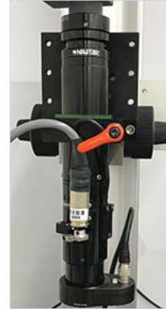
Optotune Module (Navitar 1-64805) with Zoom 6000 Motorized System
