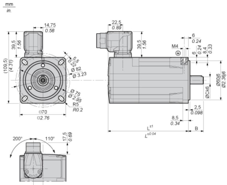
Parallel Key According to DIN 6885 A
