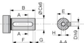
Female Thread of Shaft According to DIN 332-D
