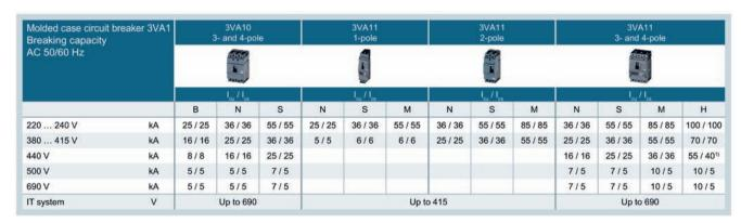
$I_n$  125 A, 160 A:  $I_{cu}/I_{cs} = 36 \text{ kA}/36 \text{ kA}$
