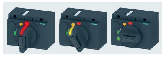
You can retrofit an active illumination kit for handling manual rotary operators. The illuminated indicator in the rotary handle signals the relevant switching position in the colors red, yellow and green. This provides clear visualization of the switching position on-site in conditions of poor visibility.
