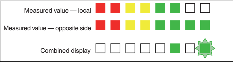
Figure 6.5 The reception level of the opposite side is greater than the reception level of the local device: green LED lights up (local device), green LED flashes (opposite side)
