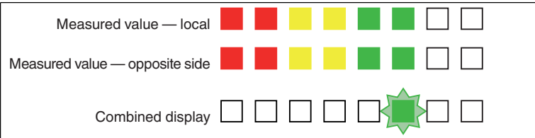
Figure 6.4 The reception level of both devices is equally good: green LED flashes (local measured value/opposite side measured value identical)
