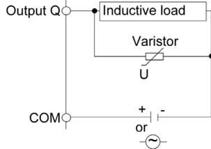
In applications where the inductive load is switched on and off frequently and/or rapidly, ensure that the continuous energy rating (J) of the varistor exceeds the peak load energy by 20 % or more.
