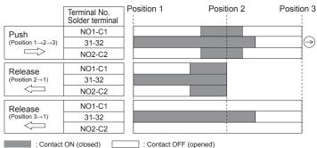
3 position enabling switch: 2 contacts; pin No.: NO1-C1, NO2-C2 Push monitor switch: 0, 1 contacts: pin No.: 31-32 (**SG-C1-21**<sub>□</sub>)
